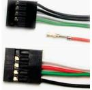
3. Working carefully so as not to damage the wires, connectors or pins, slowly reinsert the pin into the correct slot of the connector then snap closed the black tab that was lifted in step 1. Repeat these steps for each wire you need to change.
